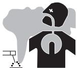
The fumes, gases and dust produced during welding are hazardous. It is mandatory to ensure adequate ventilation and/or extraction to keep fumes and gases away from the work area. An air fed helmet is recommended in cases of insufficient air supply in the workplace.
