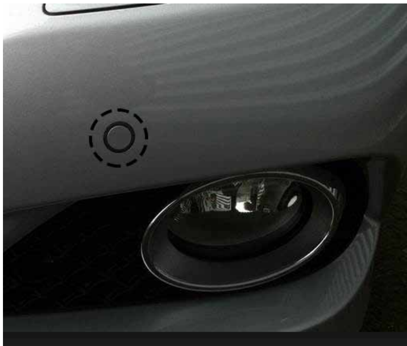
Example of parking sensor on a bumper
