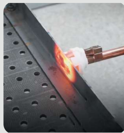
Realigning a welded assembly: - L180/Spiral inductor
