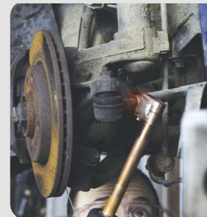
Releasing connecting rods: - Small S90 inductor - Powerduction 37LG
