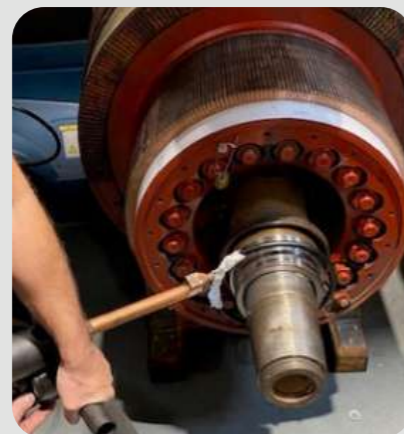
Extraction of bushings on an electric motor: - L20/D200 ring inductor - Powerduction 220LG
