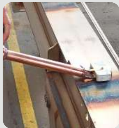
Straightening on stainless steel framework: - Large L20B4 inductor
