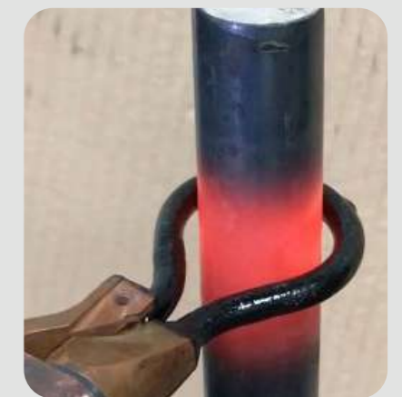
Heating a rail: - S180/D25 ring inductor
