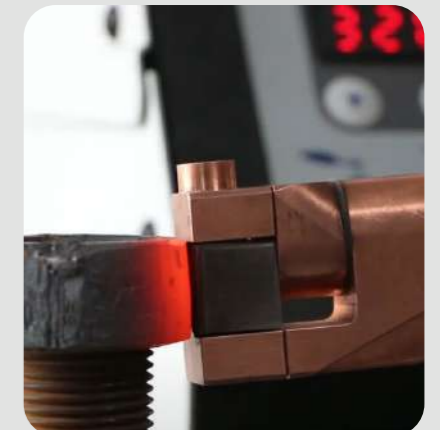
Releasing a bolt: - Small S180 inductor - Powerduction 37LG
