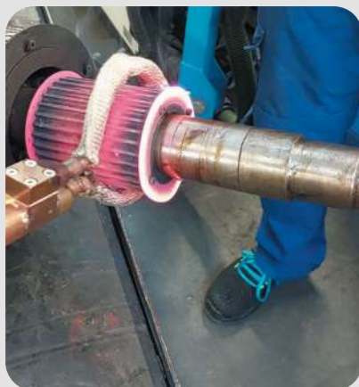
Heating a gear: - L180 ring inductor - Powerduction 220LG
