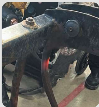
Straightening bucket teeth: - Large L20B4 inductor - Powerduction 220LG
