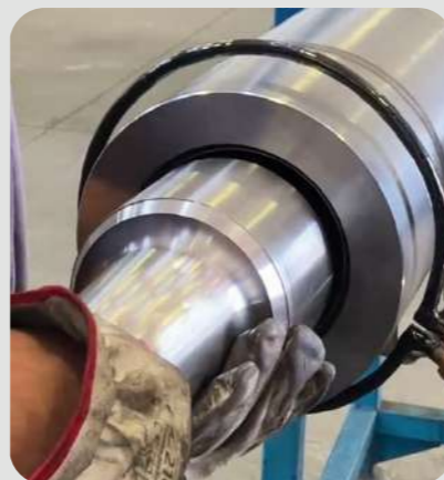
Cylinder shrink-fitting for hydraulic actuators - L20/D200 ring inductor - Powerduction 220LG
