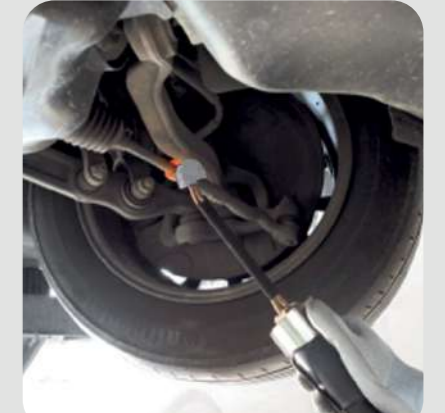
Loosening steering tie rods: - Small S20/B1 inductor
