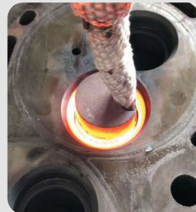
Valve seat heating: - Heat Tube inductor S180/D40 - Width Ø 40
