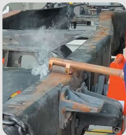
Straightening an HGV chassis: - Large L90 inductor - Powerduction 220LG
