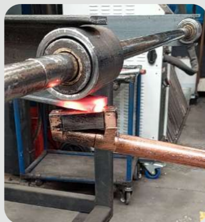
Fabrication of a trailer structure before it is welded: - Large L70 inductor - Powerduction 220LG
