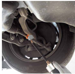
Releasing of steering linkage
