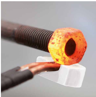
Releasing of rusted bolts
