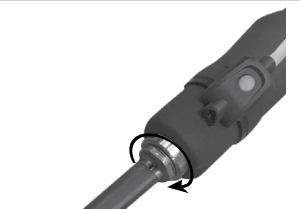
Max. tightening torque = 7 Nm
