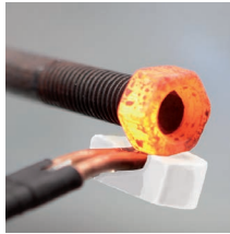
Release rusted bolts
