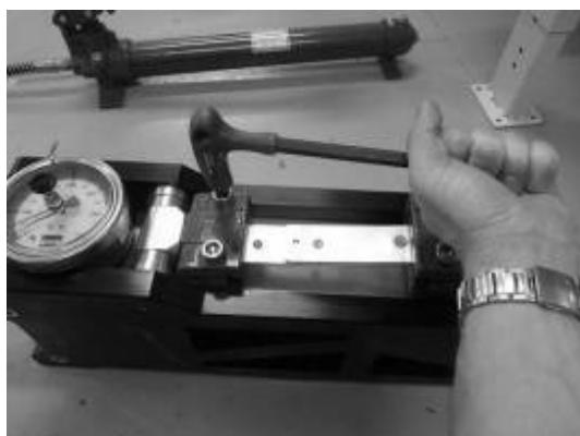
Insert the steel sheets in the jaws of the traction bench clamps. Block tightly the 4 screws using an Allen key size 10.
