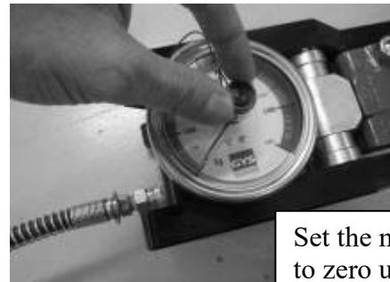
Set the maximum needle to zero using the thumb wheel on the dial.
