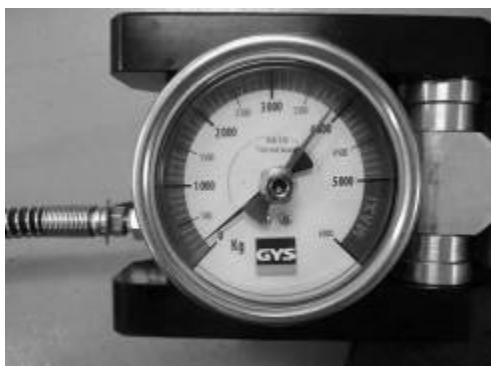
When pulling, the needles indicate the traction force. After rupture, the red needle remains at the maximum force.
