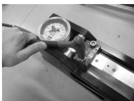
Unscrew the 4 screws of the clamps. A new pulling test can be performed.
