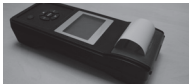
C. Place a small length of paper from the compartment and push the transparent cover to close.
